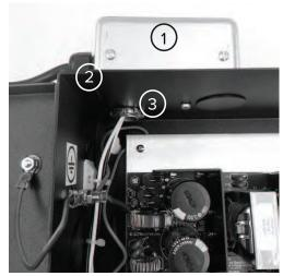
**KEY:**1 is a sample high voltage junction box, while 2 and 3 are sample cable glands.
