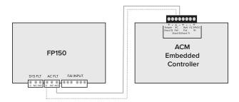
5. Starting from the ACM Embedded Controller's P3\RS-485 Port1 terminal block, connect the A, B, and Shield connections to the V100 P9\RS-485 subpanel A, B, and Shield connections as shown below (22 AWG).
