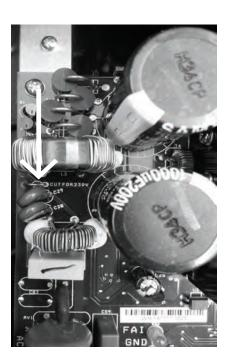
2. Ensure DC output switch is set to 24V (as shown below).
