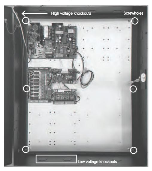
7. Setup the high voltage junction box (or equivalent), as required. Attach an appropriate cable gland to the junction box and feed the three AC wires through.
