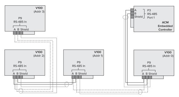
NOTE: On the V100s make sure to use the RS-485 In; avoid using the RS-485 Out.
