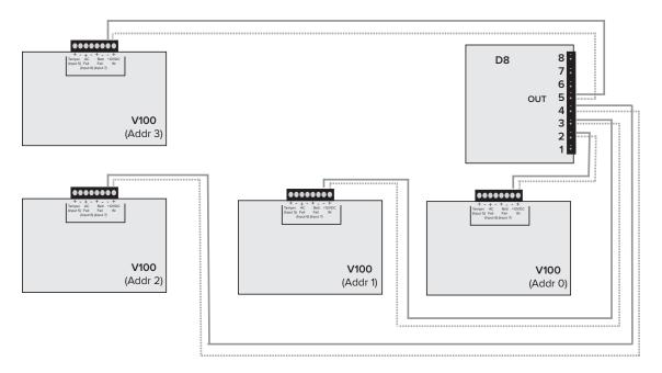
**Note**: For the steps below ensure that the card reader, door monitor (if available), request-to-exit (if available) and lock wiring from the door are fed into the power supply enclosure and route to the corresponding port on each V100 as desired.
