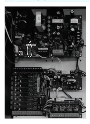
**NOTE:** On the FPO150 PSU the AC light (green - see 1 above) should be on and all warning lights (see 2 above) should be off.
