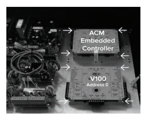
7. Mount the other V100 subpanels on the pre-installed studs mounted on the door as shown below (the arrows in the picture below show Hex nuts that will connect to the studs).
