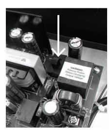
3. Connect the inputs on the FAI (Fire Alarm Input) to the building's fire alarm system, as required. See the FPO Quick Start Manual (page 3 – FAI Input Usage) for more detail. Further information is available at: http://lifesafetypower.com/docs/im\_fpo.pdf.
