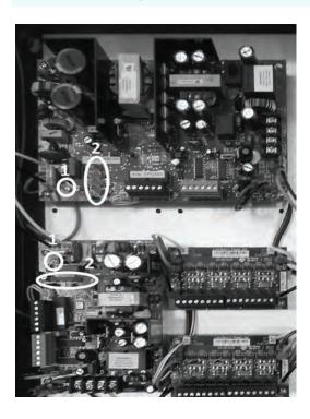
**NOTE:** On the FPO250 (on the top above) and FPO75 (below the FPO250) PSUs the AC light (green - see 1 above) should be on and all warning lights (see 2 above) should be off.
