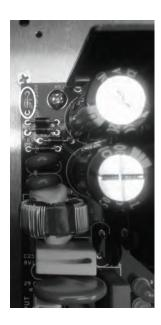
2. Ensure the DC output jumper is set to 12V (as circled below).
