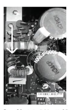
2. Ensure DC <u>output</u> switch is set to 24V (as shown below).
