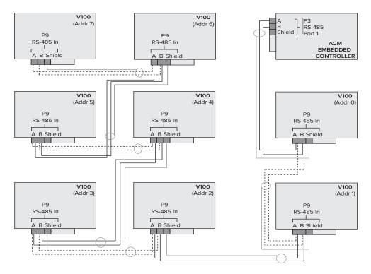
NOTE: On the V100s make sure to use the RS-485 In; avoid using the RS-485 Out.
