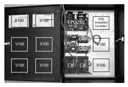
Install the ACM Embedded Controller and V100 subpanels as shown below:
