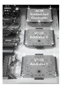
5. Mount the other V100 subpanels on the pre-installed studs mounted on the door as shown below (the arrow in the picture below show Hex nuts that will connect to the studs).
